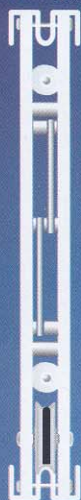
Side view of collapsible gate with a 'W' track for face and reveal fixing
